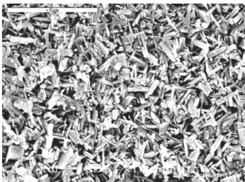
Figure 9. SEM of film deposited from \text{WCl}_6 and ethanol at 625 °C, oxidized at 400 °C for 12 h (scale bar reconstructed for clarity).
